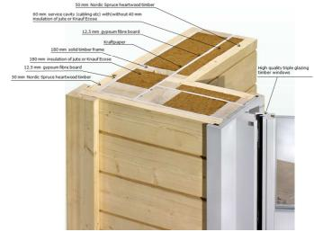
Another novelty at Stommel Haus is the new insulation material: "Thermo Jute 100" is a thermal insulation made of Jute fibres which is an adaptable material with excellent energy efficiency and sound insulation capabilities. It "snuggles" up to the timber and thus avoids sound transmission bridges.
