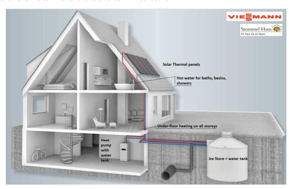
from either the ice store or solar thermal panels on the roof. The ice store also draws energy from the surrounding ground to regenerate heat.
